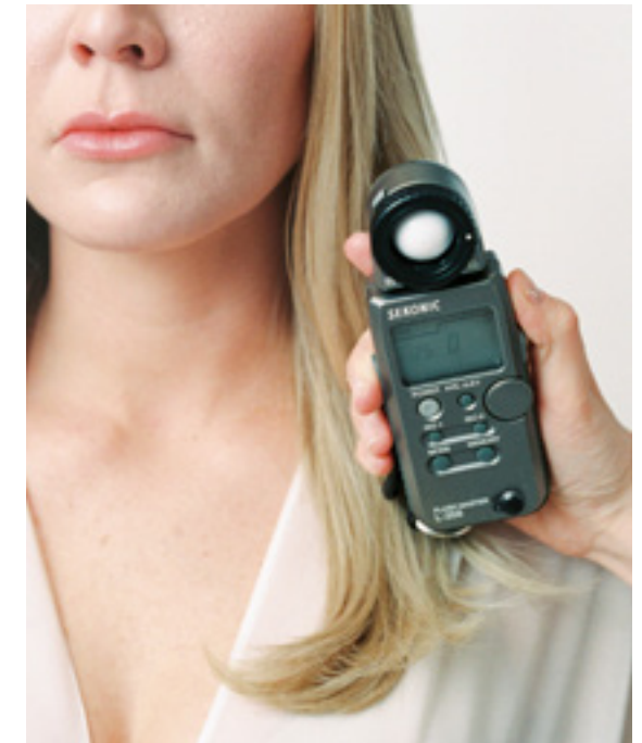
Place the light meter on the shadow side, by the person's chin, 45 degrees downward
